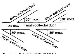
Back-draft damper kits (Part No. 3391910) are avallable from your Whirlpool dealer and should be installed in each dryer's exhaust duct to prevent exhausted air from returning into the dryers and to keep the exhaust in balance within the main exhaust duct. Unobstructed air openings are required.
